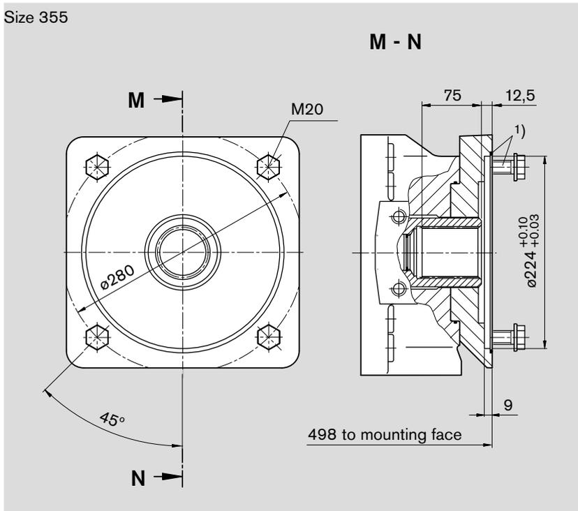
1) Mounting screws and O-ring seal are included with supply
