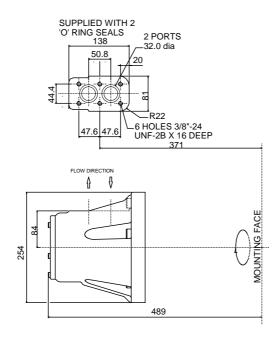
4" Valve Housing with SAE 1<sup>1</sup>/<sub>2</sub>" 4-Bolt Flanges "F4" or FM4" (see ordering code)
