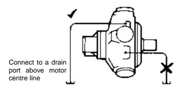
The recommended minimum pipe size for drain line lengths up to approx. 5m is 12.0mm  $^{1}/_{2}$ " bore. for longer drains, increase pipe bore to keep motor casing pressure within specified limits.
