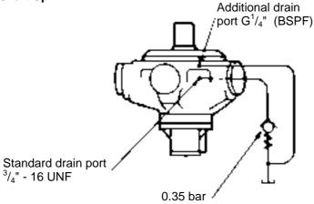
Specify "V" at model code position (3) for extra drain port,  $G^1/_4$ " (BSPF). Connect this port into main drain line downstream of a 0.35 bar check valve to ensure good bearing lubrication. Piping arrangement must not allow syphoning from the motor case. Where this arrangement is not practical, please consult Kawasaki.
